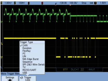
Trigger on and decode CAN serial packets.
