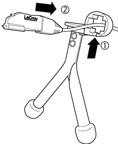
1. Slide the probe cable through the slot on the bottom of the translucent holder section.
