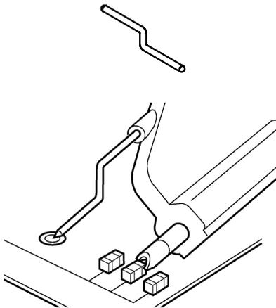
The offset pin is designed to be attached to either socket of the probe head. The offset pin is the highest quality grounding solution and is recommended in high frequency applications.
