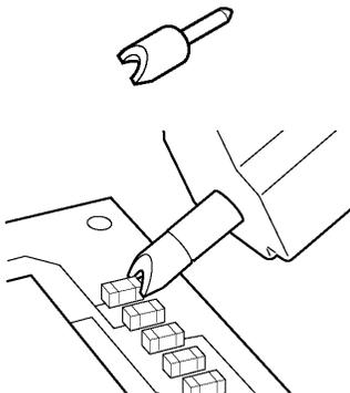
The crescent shape of this tip is designed to fit tightly on capacitors, resistors, transistors and other surface mount components with discrete leads. Fits in either probe socket.
