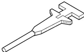
A pincher like tip designed to hold onto larger wires and components than possible with the Micro Clip, including through-hole mounted components.
