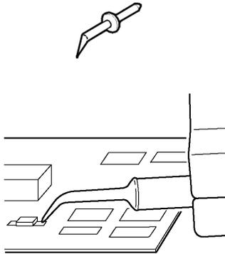
Made out of titanium, this tip is ideal for situations that require the user to hold the probe parallel to the circuit board under test. Also gives the user more control when holding the probe like a pencil. Fits in either probe socket.
