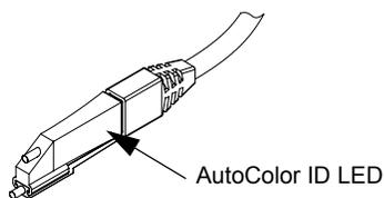
The AutoColor ID consists of an LED inside the probe head which illuminates the probe body in the default trace color of the channel to which the probe is connected.
