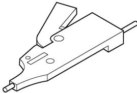
A pincher like tip designed to hold onto fine pitch leads and small components, commonly found in SMD ICs. Fits in either probe socket, or can be used with a lead.
