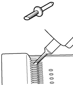
Covered in insulation on all sides (except for a small edge), this tip was designed to prevent shorting neighboring IC leads. The gold part of the tip is not insulated and should touch the IC lead to be tested. It is one-size-fits-all and will work with any IC lead pitch. Fits in either probe socket.
