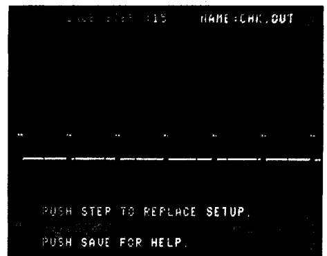
Sequences are arranged and modified with the front-panel controls. Information about the sequence steps and directions for the operator are written on the scope display for easy reference.
