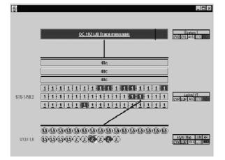
Error and alarm status clearly presented for each detected STS/AU channel, and for all VT/TU channels in a selected STS/AU.
