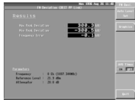
▲ DECT FM deviation measurement
