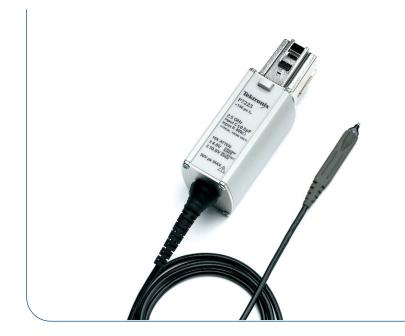
Selecting the right probe for your application is key to attaining the best signal fidelity in your measurements. Active probes provide truer signal reproduction and fidelity for high frequency measurements. With our ultra-low input capacitance and high input resistance provided by the P7225, you are able to make measurements with minimal signal distortion. This probe offers a wide 8  $V_{p-p}$  dynamic range to access today's voltage levels.
