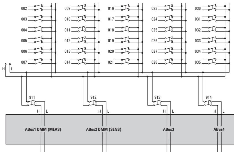
**Figure 4.** 34925A 40/80-channel optically isolated FET mux (shown in 1-wire mode bank 2)
