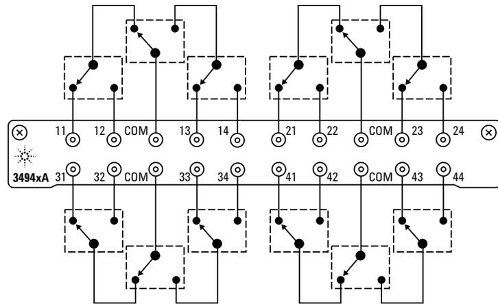
The 34941A and 34942A are configured as four independent 1x4 RF multiplexers on a single module. Multiple banks can be connected together to create a larger multiplexer—up to 97 RF multiplexer channels in a single 34980A mainframe. To prevent ground loops, individual multi-
