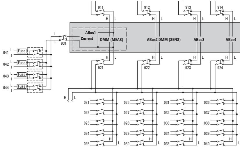
Multiple multiplexers can connect to the built-in analog buses, allowing you to scan up to 560 2-wire channels or 640 1-wire channels in a single mainframe. The 34921A also offers 4 channels for directly measuring current. Or if you need more current channels, shunts can be added to the terminal block for easy current measurements.
