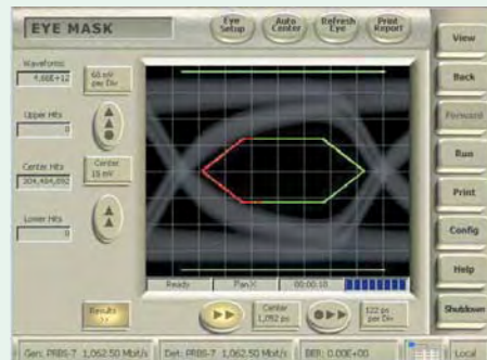
Industry standard and custom masks are tested many times faster using BER-based methods built into the BA1500.
