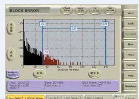
Block error statistics are often more important to system operation than exact bit error measurements. Block sizes can be adjusted and histograms show how many times blocks occur with different numbers of errors in them.
