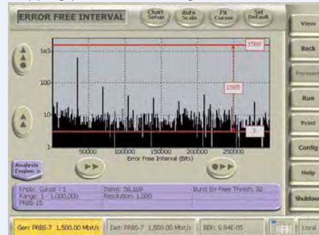
Error free intervals that are repetitive are a sure sign of a systematic error. Finding spikes such as these during a measurement can quickly indicate the interfering frequency.
