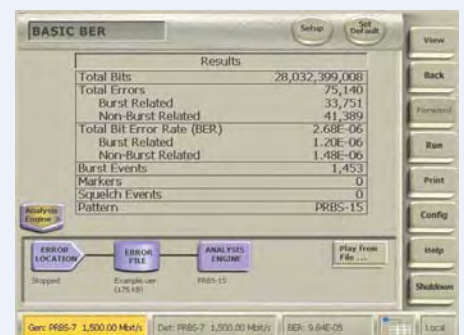
The individual error rates and counts for bit versus burst errors are displayed on the Basic BER view. This simple separation can focus debugging efforts in the right area.
