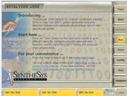
The Home view is the starting point for the BA1500. The touchscreen buttons on the right-hand side are used to select the view, operating mode, and configuration of the analyzer.
