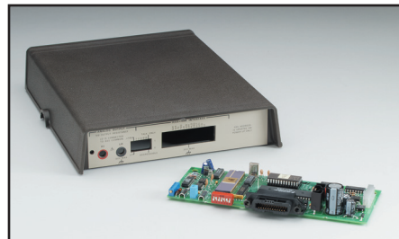
Model 5802: Isolated analog output/IEEE-488 interface for Model 580 (cover included).
