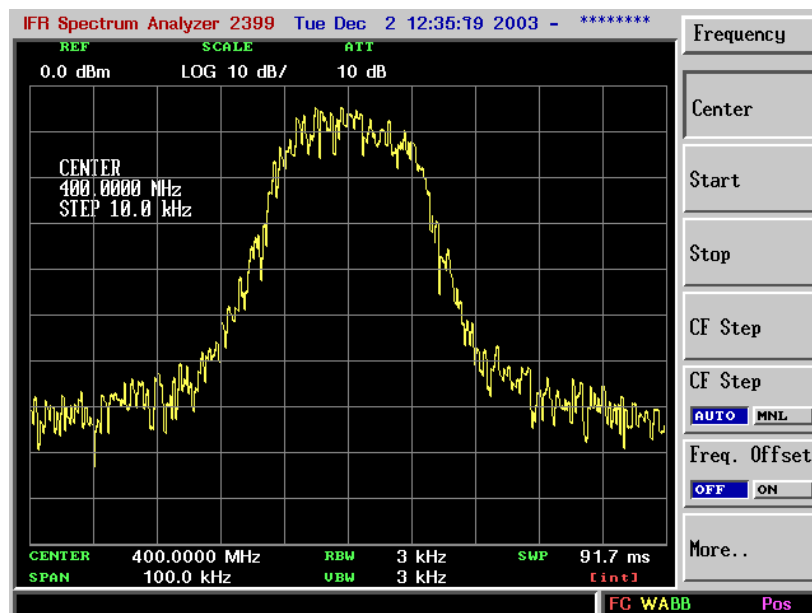
Fig. 6-10 Spectrum analyser display showing \pi/4 DQPSK modulated carrier
