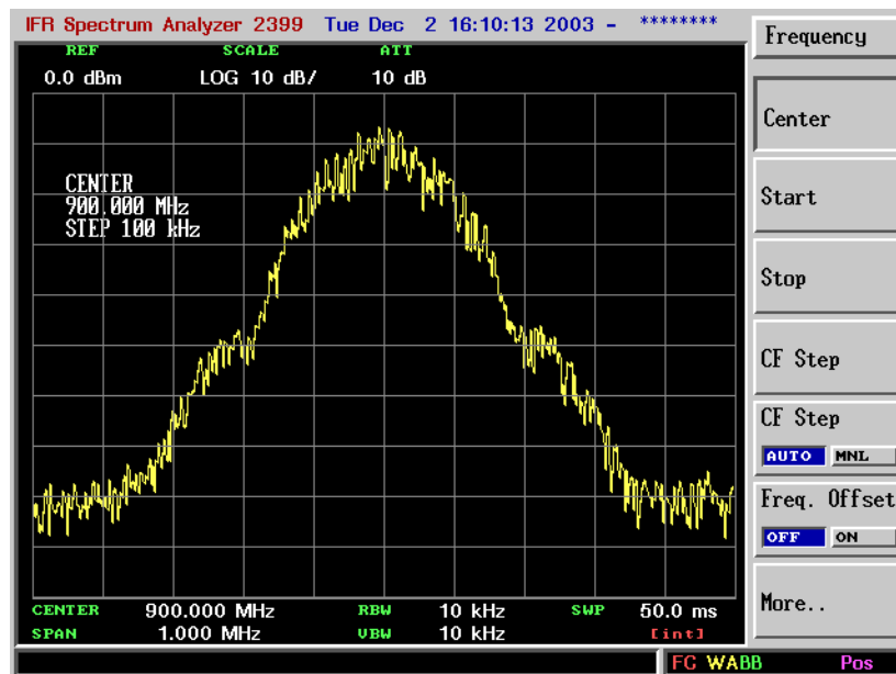
Fig. 6-12 Spectrum analyzer display showing GMSK modulated carrier
