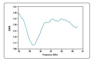
Typical SWR, 33 GHz to 50 GHz (25 °C  $\pm 10$  °C) for N8486AQ power sensor
