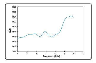
Typical SWR, 100 kHz to 6 GHz (25 °C  $\pm$ 10 °C) for N8482B power sensor
