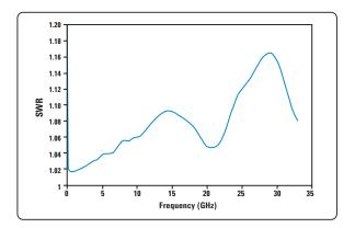
Typical SWR, 10 MHz to 26.5 GHz (25 °C $\pm$ 10 °C) for N8485A sensor
