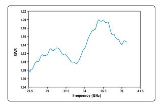
Typical SWR, 26.5 GHz to 40 GHz (25 °C ±10 °C) for N8486AR power sensor
