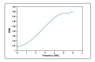
Typical SWR, 100 kHz to 6 GHz (25 °C  $\pm 10$  °C) for N8482H power sensor
