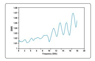
Typical SWR, 10 MHz to 18 GHz (25 °C  $\pm$ 10 °C) for N8481B power sensor
