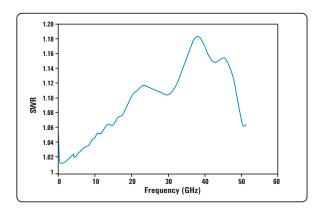
Typical SWR, 50 MHz to 50 GHz (25 °C ±10 °C) for N8487A power sensor
