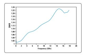
Typical SWR, 10 MHz to 18 GHz (25 °C  $\pm$ 10 °C) for N8481H power sensor
