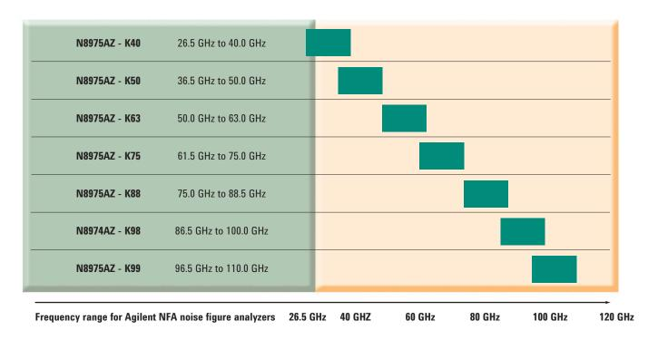
**Note:** The K-Series block downconverters can only be used with the N8975A and N9020A MXA signal analyzers.
