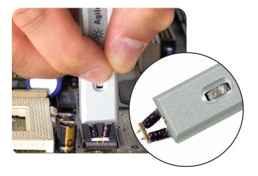
• N5439A ZIF probe head provides 28 GHz bandwidth in an economical replaceable tip form factor. Because of their extremely low loading, the ZIF tips can be left on the DUT as the probe head is moved from one probing site to the next. Order N5440A (450  $\Omega$ ) or N5447A (200  $\Omega$ ) for a set of 5 ZIF tips with plastic sporks to aid in soldering the tips to your DUT. Variable spacing from 5 mil – 80 mil (or 0.127 mm – 2 mm).
