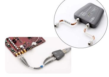
• N5441A solder-in probe head is an economical, semipermanent connection that provides up to 16 GHz of bandwidth. Variable span of the leads ranges from 5 mil - 80 mil (or 0.127 mm - 2 mm).
