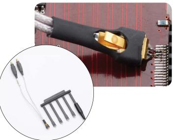
N5444A 2.92 mm/3.5 mm/SMA probe head (28 GHz) allows you to connect two 2.92 mm, 3.5 mm or SMA cables to make a differential measurement on a single oscilloscope channel. Order N5448A 2.92 mm head flex cables (10" or 25 cm) to extend the cable length and add convenience.
