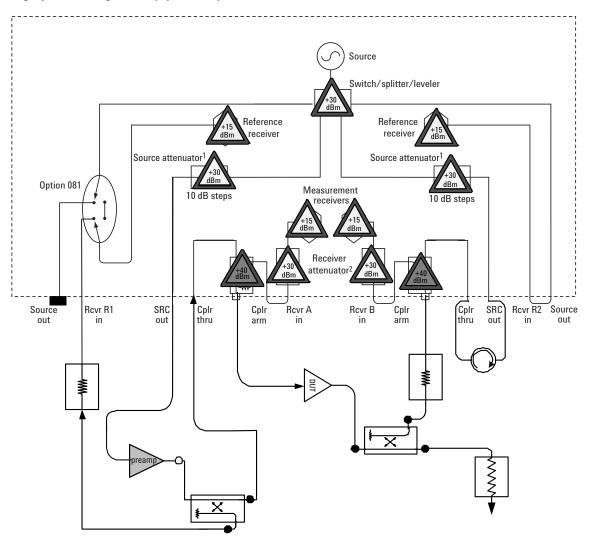
Power levels shown on the diagram are damage levels. At a minimum, keep power levels 6 dB below damage level. For optimal performance, keep the power level incident upon the receivers -20 dBm or less. This will keep the receivers out of compression.
