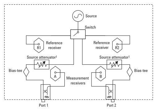
1. Source attenuator for E8362/3/4B is 60 dB in 10 dB steps. Source attenuator for E8361A is 50 dB in 10 dB steps.
