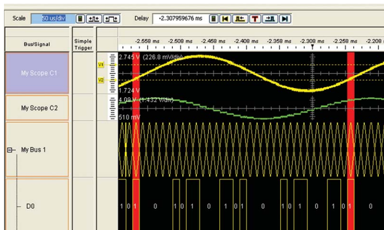
Figure 10. Gain quick insights into event frequency throughout a trace by using the color selection in the Filter tool. Advanced filtering capabilities of data record. Shown here is a data write value of D5 on My Bus 1 and voltage level range of 2 to 2.5 V.
