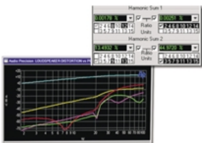
Harmonic selection controls and graph of individual harmonic amplitude versus frequency.
