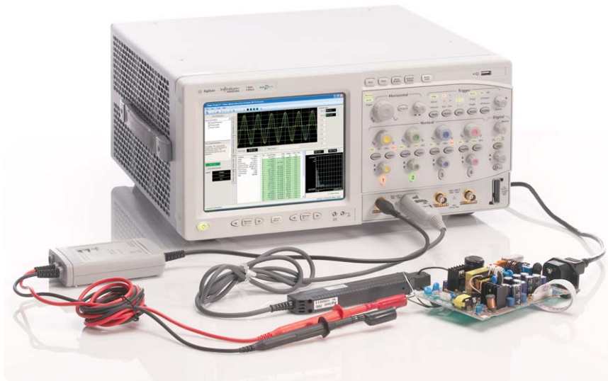
Figure 1. Power measurement application running on an Agilent 8000 Series oscilloscope provides a single-box solution for testing switching mode power supply characteristics.
