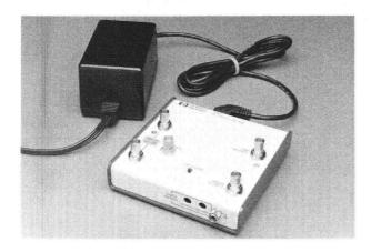
The HP 1133A TV/Video Sync Pod is an accessory that provides users with TV sync triggering for most analog or digitizing oscilloscopes. It features clamped or undamped video outputs that can be viewed on the oscilloscope's vertical channels and trigger outputs that can synchronize the oscilloscope to video frame and individual lines.
