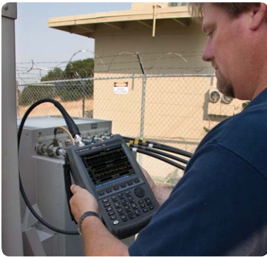
Perform and view return loss and distance to fault measurements at the same time
