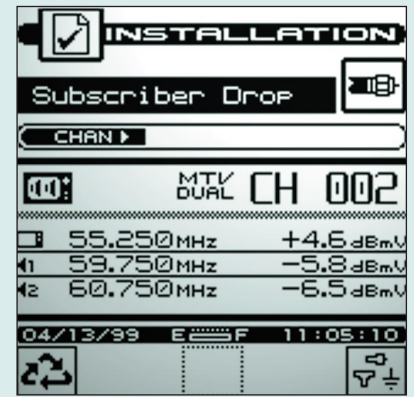
Pressing the cycle soft key provides a detailed view of what specific error is on the specific channel
