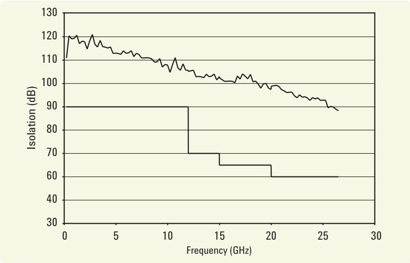
Figure 12. Agilent L Series multipoint switch isolation versus frequency
