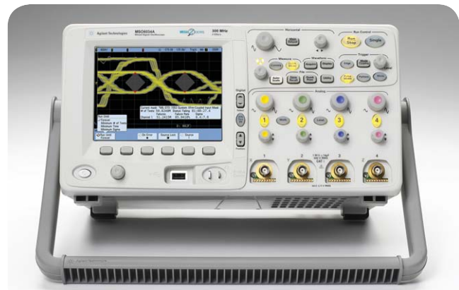
Figure 13. Agilent's 6000 Series oscilloscopes are available with a battery option for remote/field testing of MIL-STD 1553 applications.
