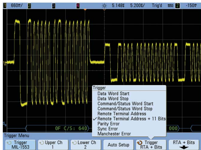
Figure 2. Trigger on specific MIL-STD 1553 communication words and errors.
