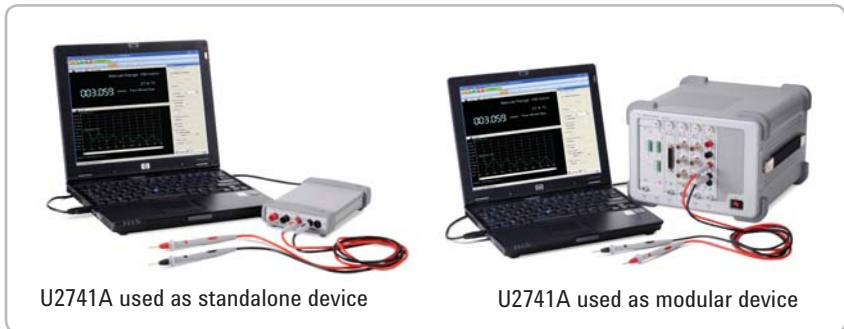
Figure 1. The U2741A DMM showing dual-play capability
