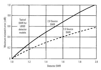
Figure 4. Measurement uncertainty due to detector source mismatch
