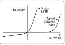
Figure 1. Diode V/I characteristics
