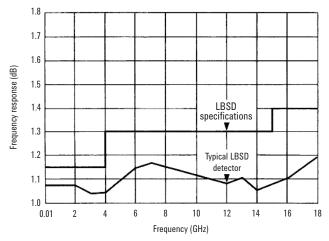
Figure 3. Detector SWR specifications
