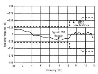
Figure 2. Detector frequency response specifications
