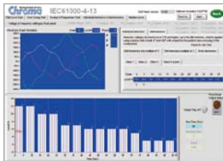
Voltage Harmonic & Interharmonic Test
