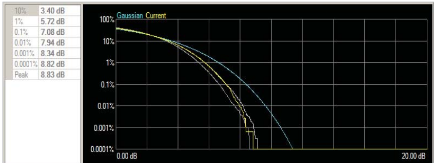
Figure 2b. CCDF plot of 10 MHz enhancement uplink LTE-Advanced carrier
