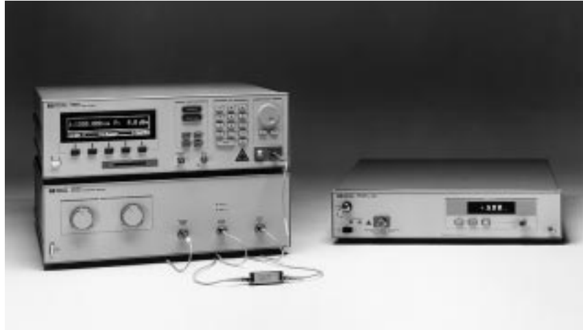
Figure 5. Polarization mode dispersion measurement setup using the HP 8509B and HP 8168 or HP 83424 lightwave sources.
