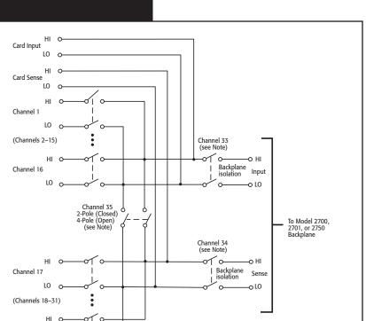
Channels 33–35 in this schematic refer to the designations used for control and not actual available channels.
