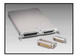
The Model 7709 plug-in module is a two-pole, 6×8 matrix module. It can connect any combination of six differential channels of instrumentation to any combination of eight differential device-under-test channels. The instrumentation can be AC and DC sources, internal or external meters, oscilloscopes, etc. This matrix configuration allows wide flexibility for complex test systems.
