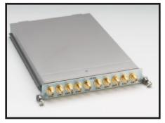
The Model 7711 plug-in module provides an economical, wideband signal routing solution that complements the DC/low frequency switching and measurement capability of the Integra Series
