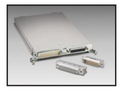
The Model 7707 plug-in module offers 10 channels of 2-pole or 5 channels of 4-pole multiplexer switching that can be configured as two independent banks of multiplexers. The Model 7707 also provides 32 digital input/output channels (four 8-bit ports) for I/O control. Connect the Model 7707 to industry standard solid-state relays to switch up to 980VA.
