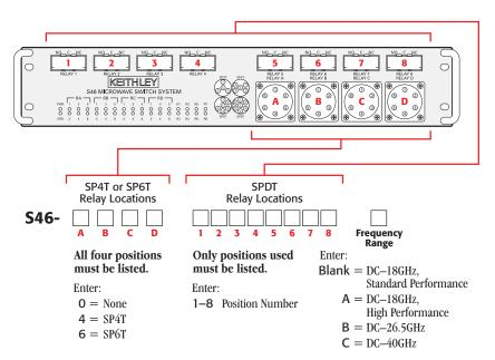
**Multipole relay locations A–D:** Enter a "4" for an SP4T relay or a "6" for a SP6T relay in the required location. Enter a "0" in unused multi-pole locations. There must be digits in all four positions.
