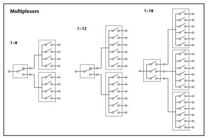
$\textbf{MAXIMUM CONFIGURATION:} \ (8) - \textbf{Unterminated SPDT relays.} \ (4) - \textbf{Unterminated multi-pole relays} \ (8P4T, SP6T).$
