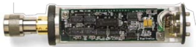
An EEPROM in all Giga-tronics sensors automatically applies the correct cal factor, so you save time and avoid measurement errors.
