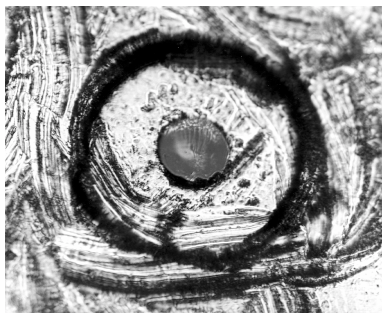
Figure 3-6. Damage from improper cleaning.
