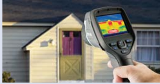
Infrared cameras quickly locate moisture related problems
