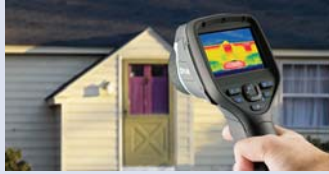
Infrared cameras quickly locate moisture related problems
