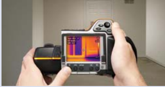
Infrared cameras quickly locate moisture related problems
