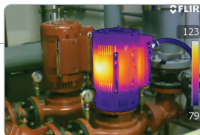
Fused thermal images insert IR image set within a temperature interval onto corresponding digital image.
